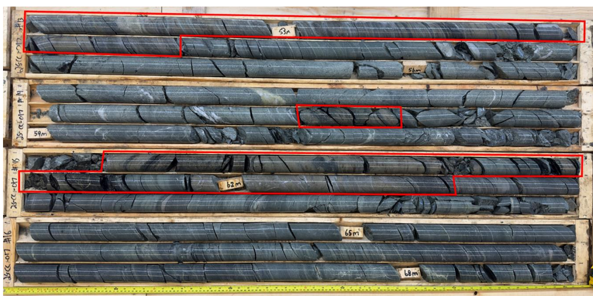
Figure 1. Hole 25-CC-017 from 52.25m to 68.4m. Intervals of Semi-Massive pyrite mineralization are outlined in red.
