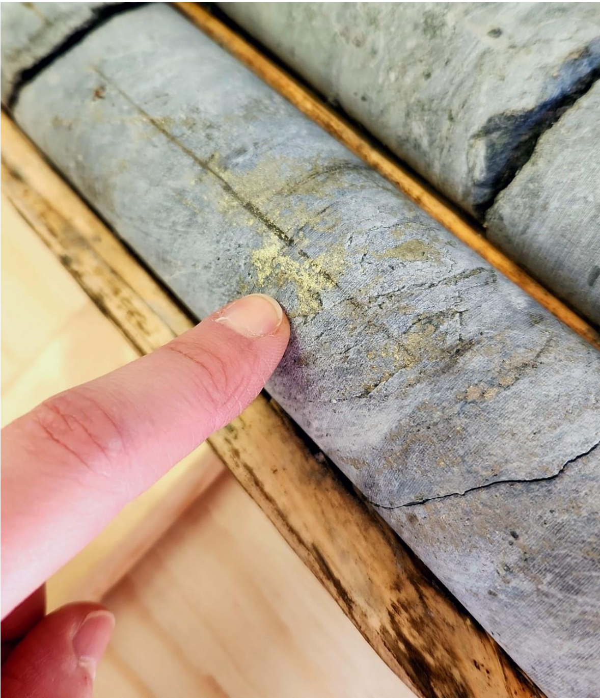
Image 1: Interpreted chalcopyrite mineralization at 19m downhole length in hole 25-CC-001, Copper Creek project, Baie Verte
