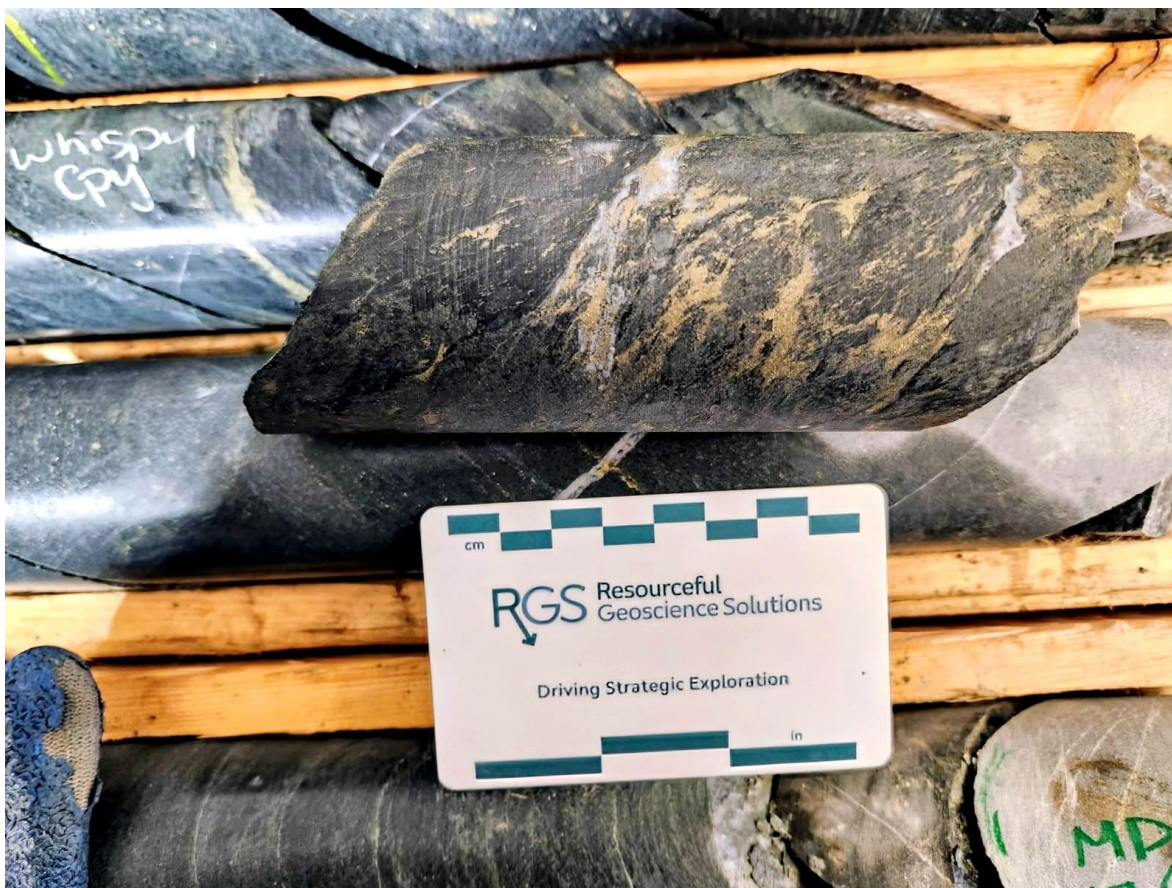
Image 2: Interpreted chalcopyrite mineralization at 15.75m downhole length in hole 25-CC-002, Copper Creek project, Baie Verte
