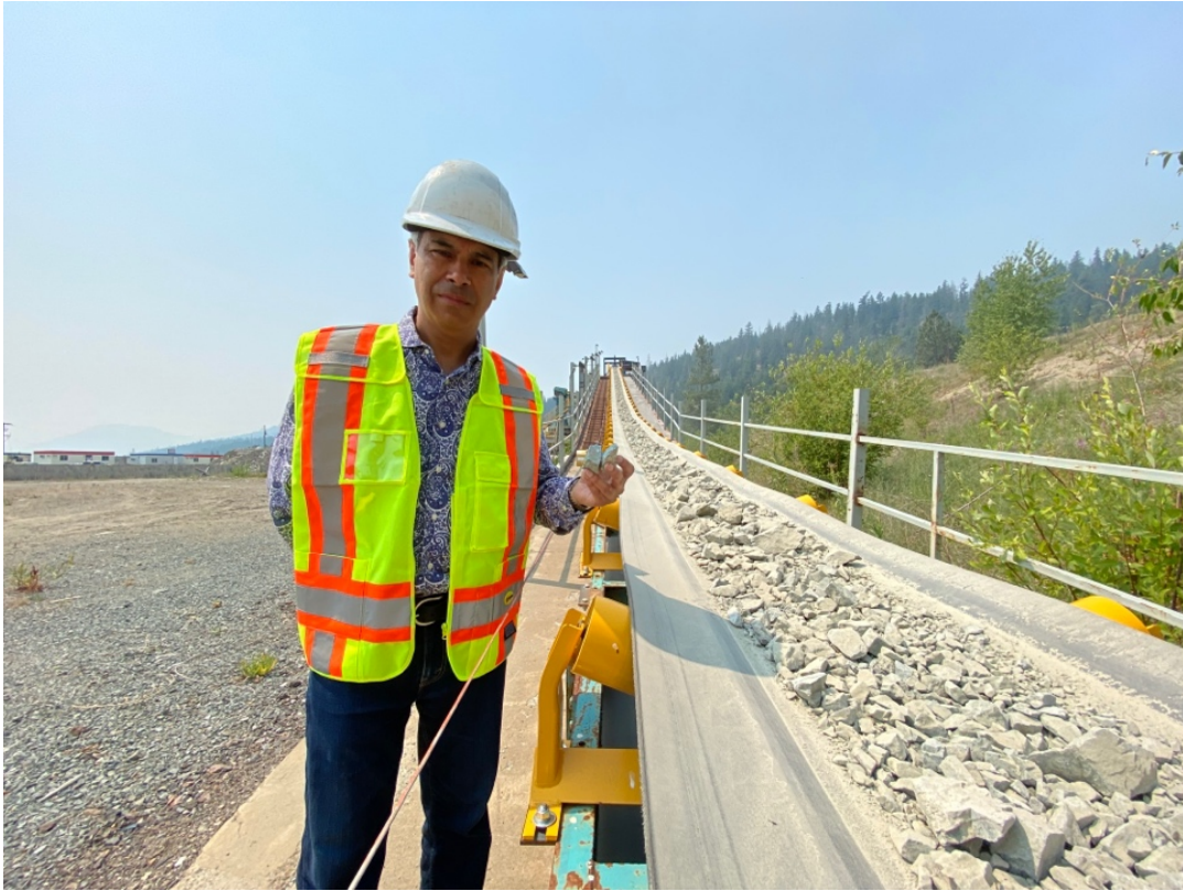
Blue Lagoon Resources President & CEO, Rana Vig, standing next to conveyer transporting Dome Mountain mineralized material from Nicola's primary crusher to its secondary crusher during testing phase in 2021
