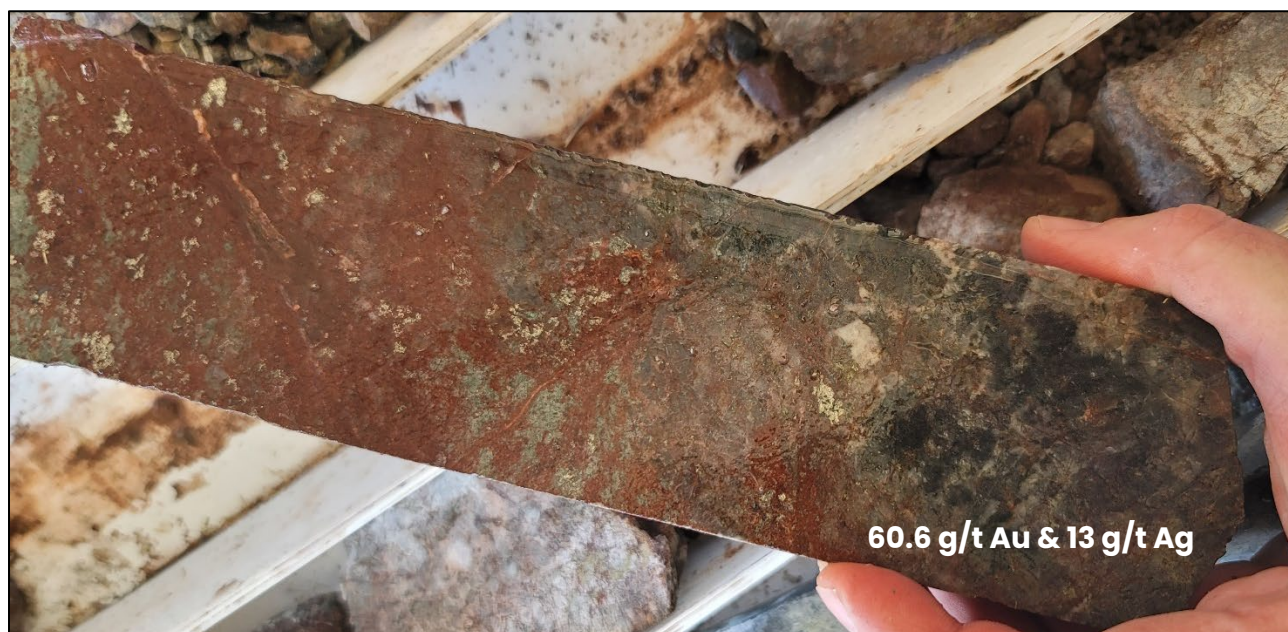
Photo 1. Close up of high-grade gold sample (JES-25-104, 1.6 meters of 60.6 g/t Au and 13 g/t Ag, from 87.8m depth vertically from surface). Local faulting and associated intense hematite and silica alteration have replaced the original andesite host rock. This style of mineralization has been recorded across the Main Zone at surface and in drill core.
