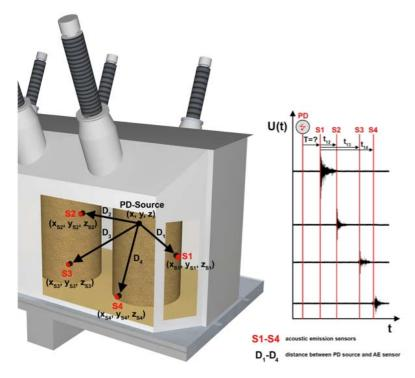
MAST patented sensors are located in the critical areas of a transformer, directly in the oil and are designed to detect the partial discharge event, measure the severity of the partial discharge and locate it accurately so as to inform the user of the root cause of the partial discharge and how to direct their maintenance effort.
