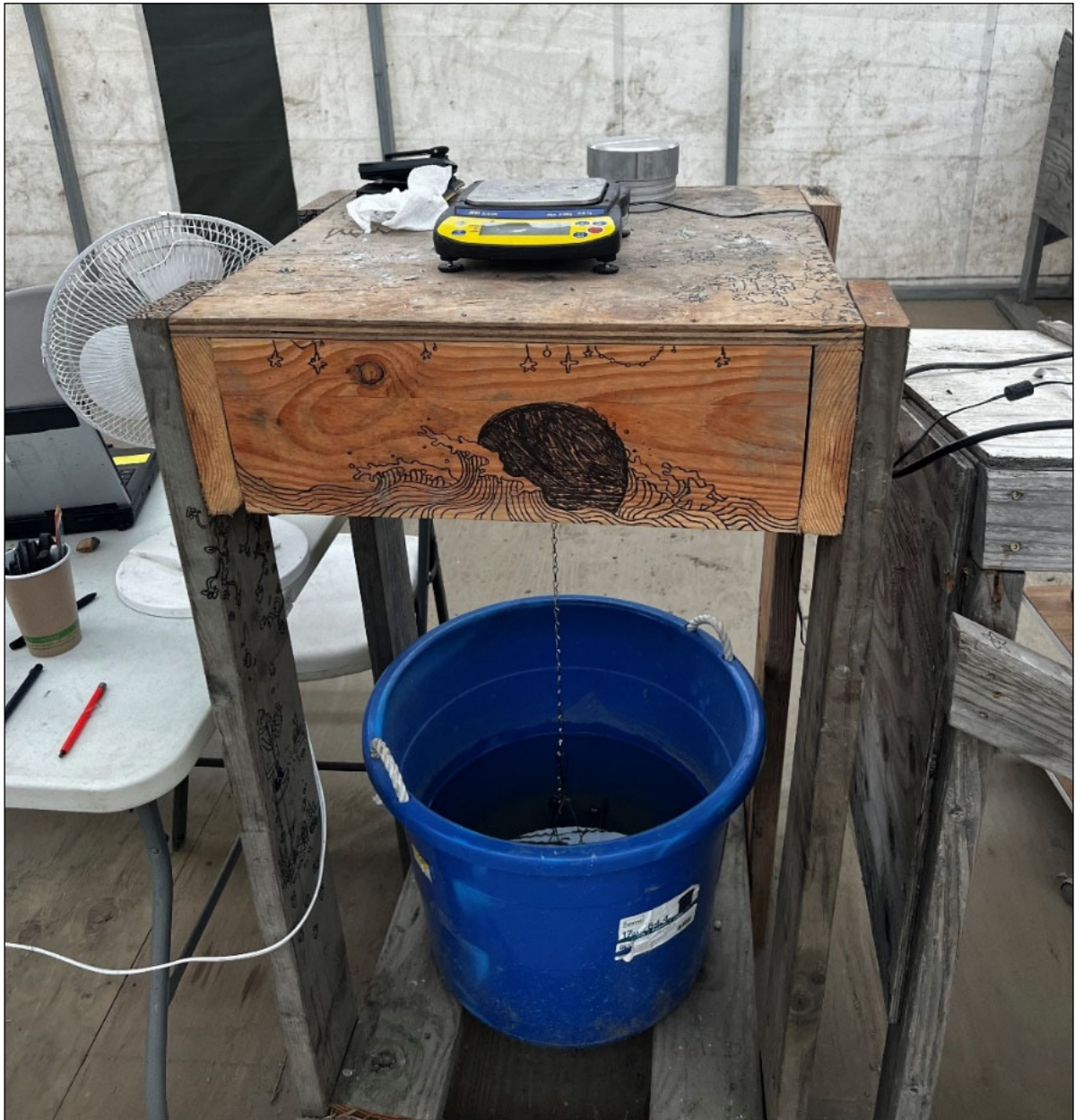
Figure 10-4: Specific Gravity Measurement Setup at Palmer
