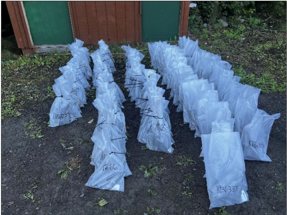
Figure 12-3: Core Samples Cut and Prepared for Sample Submission
