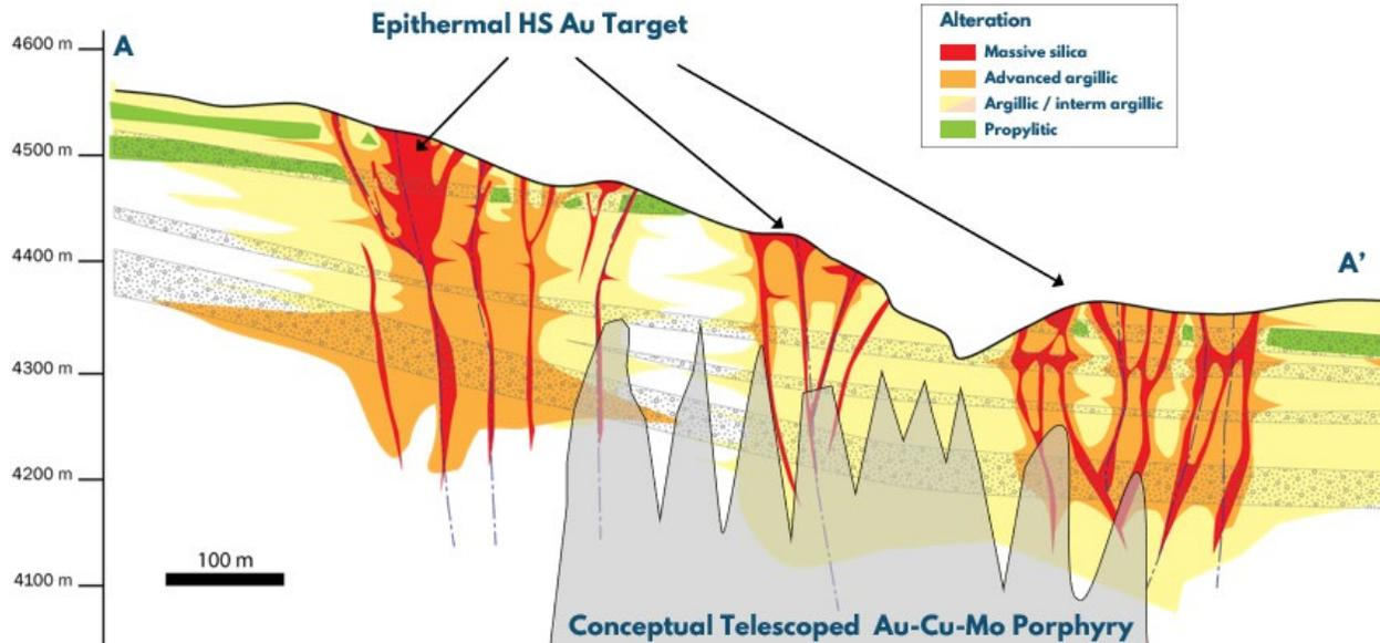
Figure 2 – Proposed Geological Model Along Section Line A-A' in Figure 1 (Looking NE) with High Sulphidation Epithermal Gold and Porphyry Copper-Molybdenum Targets.
