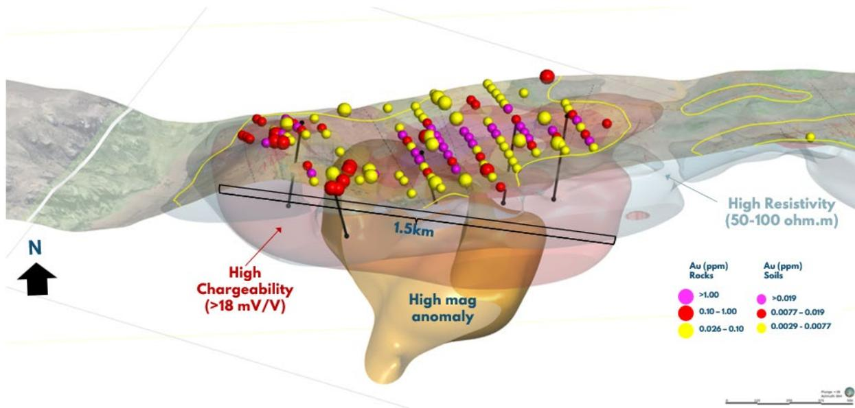
Figure 3 – Proposed Drill Program – Gold Geochemistry Imposed on the 3D Inversions of IP Chargeability-Resistivity and Magnetic Susceptibility Geophysical Data.
