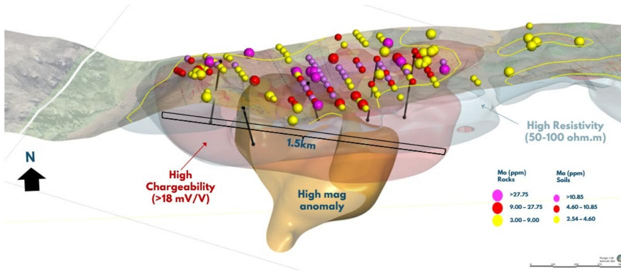
Figure 4 - Proposed Drill Program – Molybdenum Geochemistry Imposed on the 3D Inversions of IP Chargeability-Resistivity and Magnetic Susceptibility Geophysical Data.
