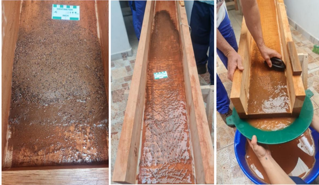
Figure 63. The fine material was washed, the coarse material was collected in a pan to improve the concentration of heavy material.
