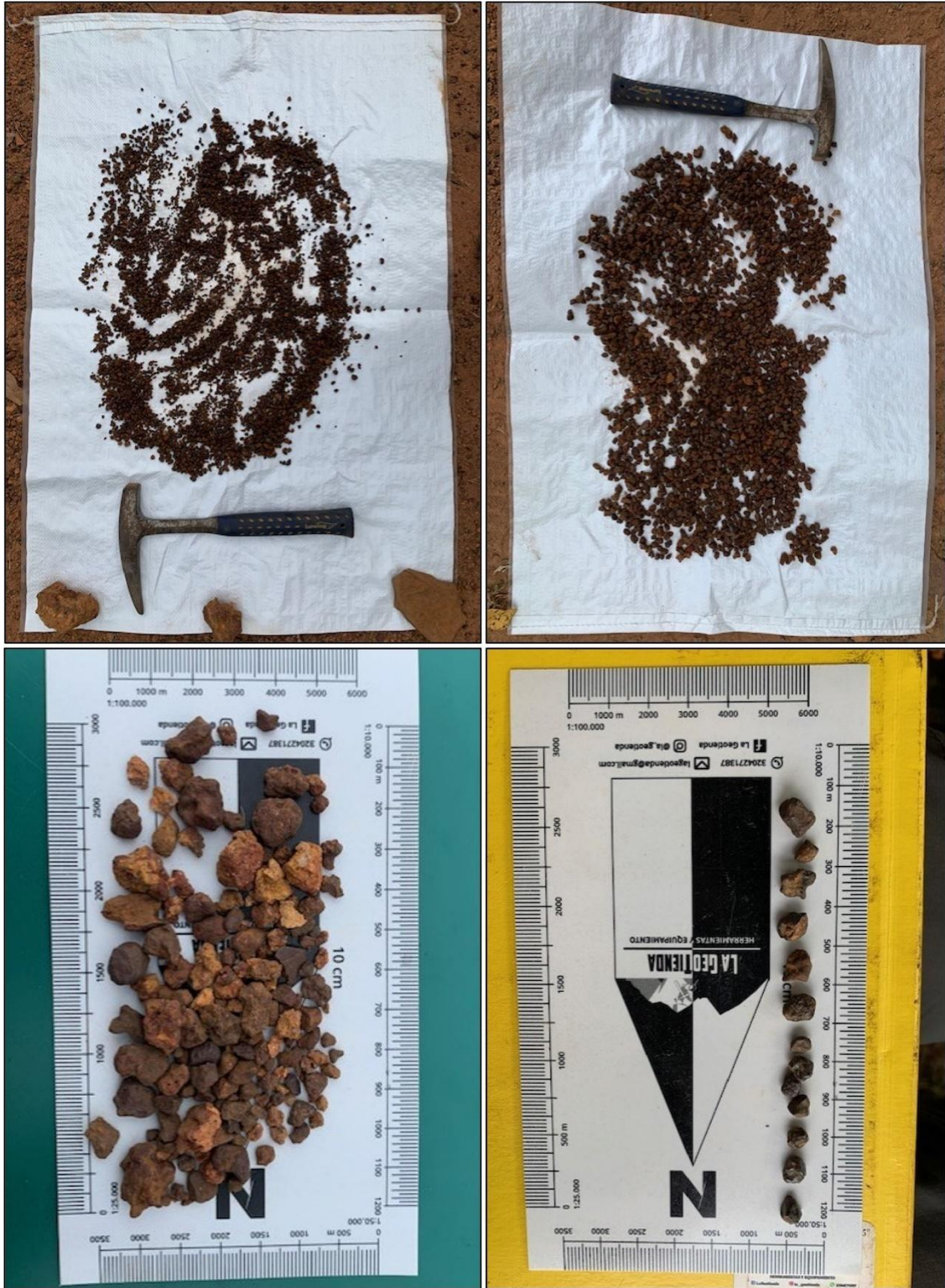
Figure 21. Grain size scale of Hematite nodules present in the iron oxides rich zone.
