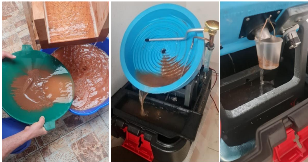
Figure 65. Coarse material from wood channel was re-concentrated in an automatic concentrator.
