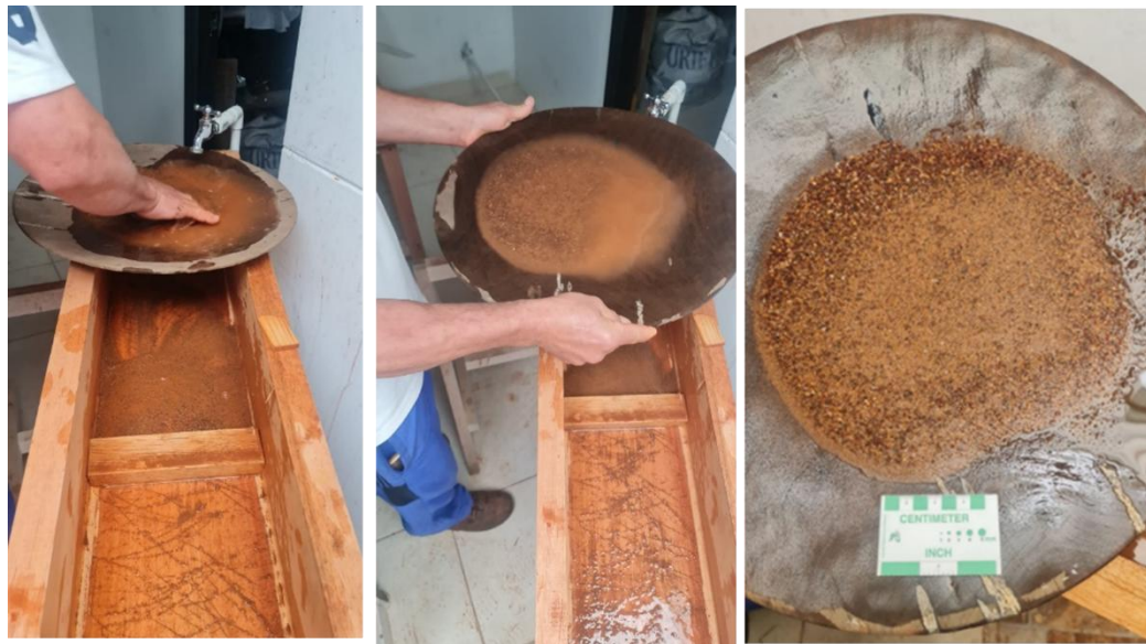
Figure 64. Fines cleaning using a pan to concentrate the heavy material.
