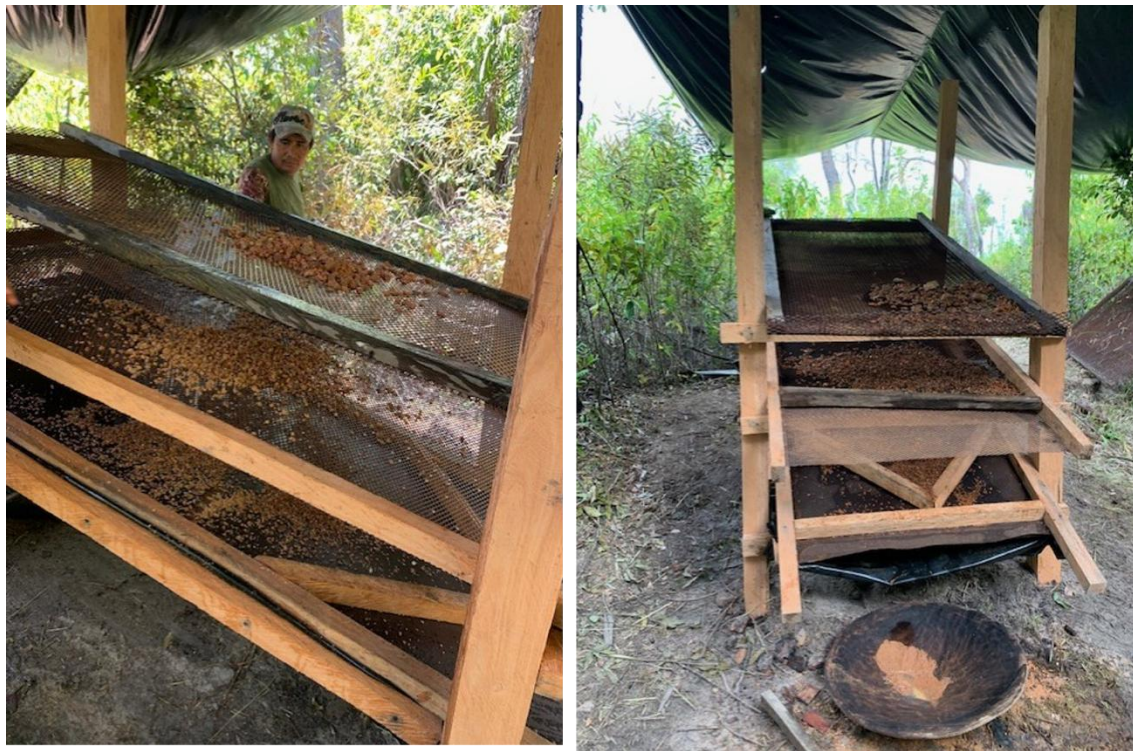
Figure 58. Separation of particle sizes by sieves with +3/8, -3/8 + 1/8, -1/8 mesh.
