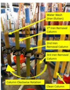
Figure 1.2 - REE separation system based upon a continuous ion exchange process (CNW Group/Lithos Energy Ltd.)
