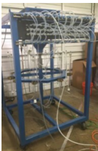
Figure 1.1 - REE separation system based upon a continuous ion exchange process (CNW Group/Lithos Energy Ltd.)
