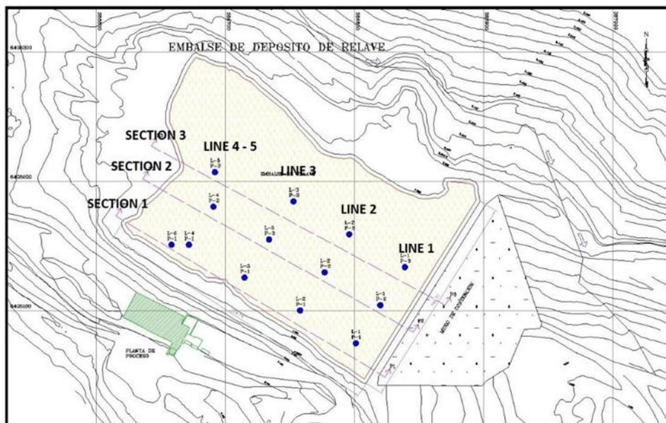
Figure 7. Tailings pond with wells drilled in sections and lines.
