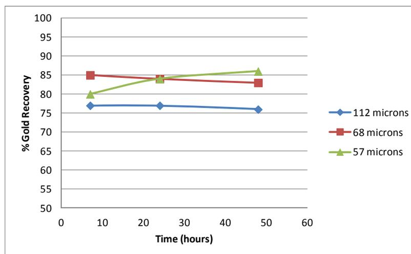
**Figure 1 – Omega Composite Whole Ore CN Recovery vs. Time and Grind Size**
