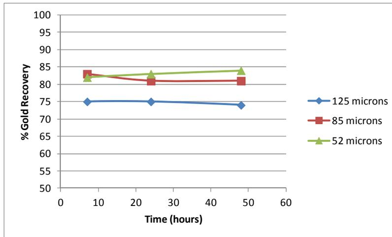
**Figure 2 – Omega Composite Gravity Tailing Recovery vs. Time and Grind Size**
