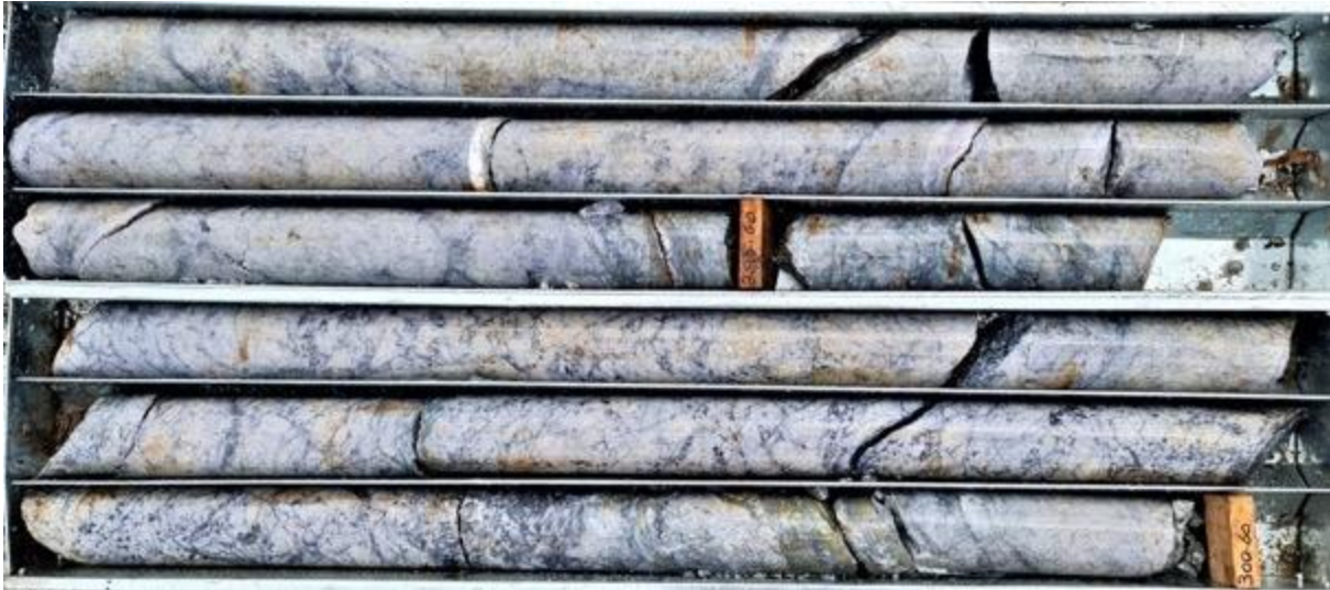
Figure 7. CDH003: mineralized quartz diorite porphyry with dominant bornite and lesser chalcopyrite
