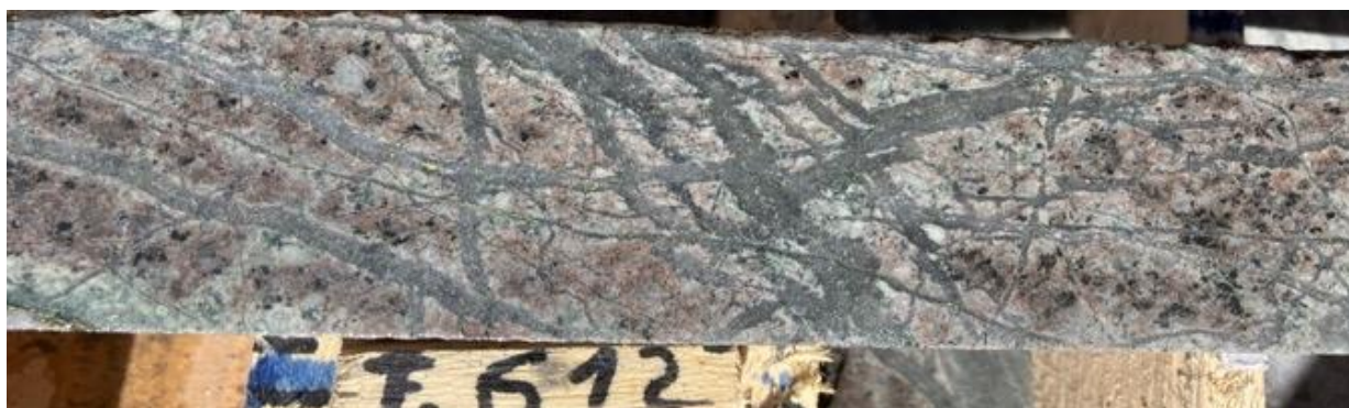
Figure 3. PIU-03-2024DDH Intense porphyry A type quartz vein stockwork with disseminated chalcopyrite and late veins associated with intermineral potassic (Kfeldspar-quartz) alteration
