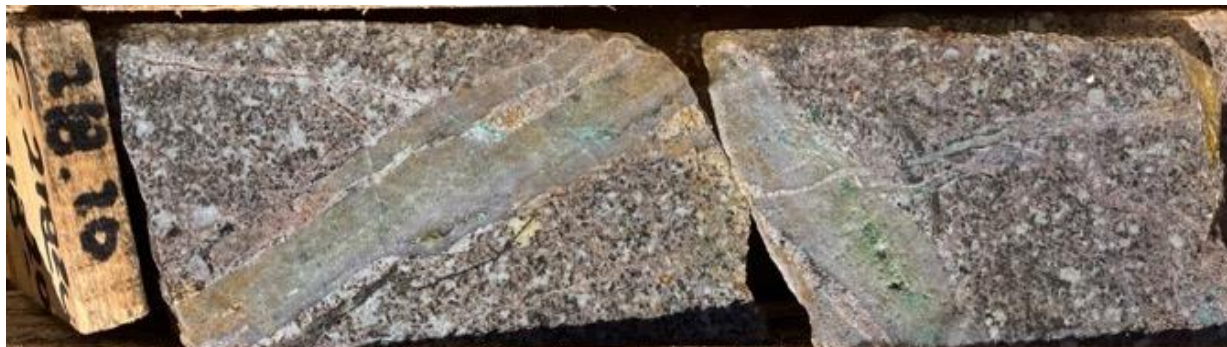
Figure 2. PIU-03-2024DDH Disseminated copper oxides in porphyry A-type quartz veinlets overprinting early biotite-magnetite altered quartz-diorite porphyry
