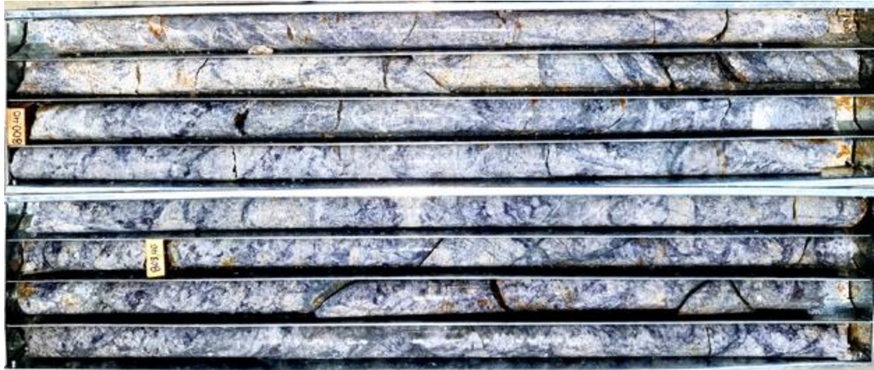
Figure 6. CDH001: Quartz diorite with siliceous-phyllitic alteration overprinted on potassic alteration, brecciation and considerable disseminated bornite in a dark gray silica matrix
