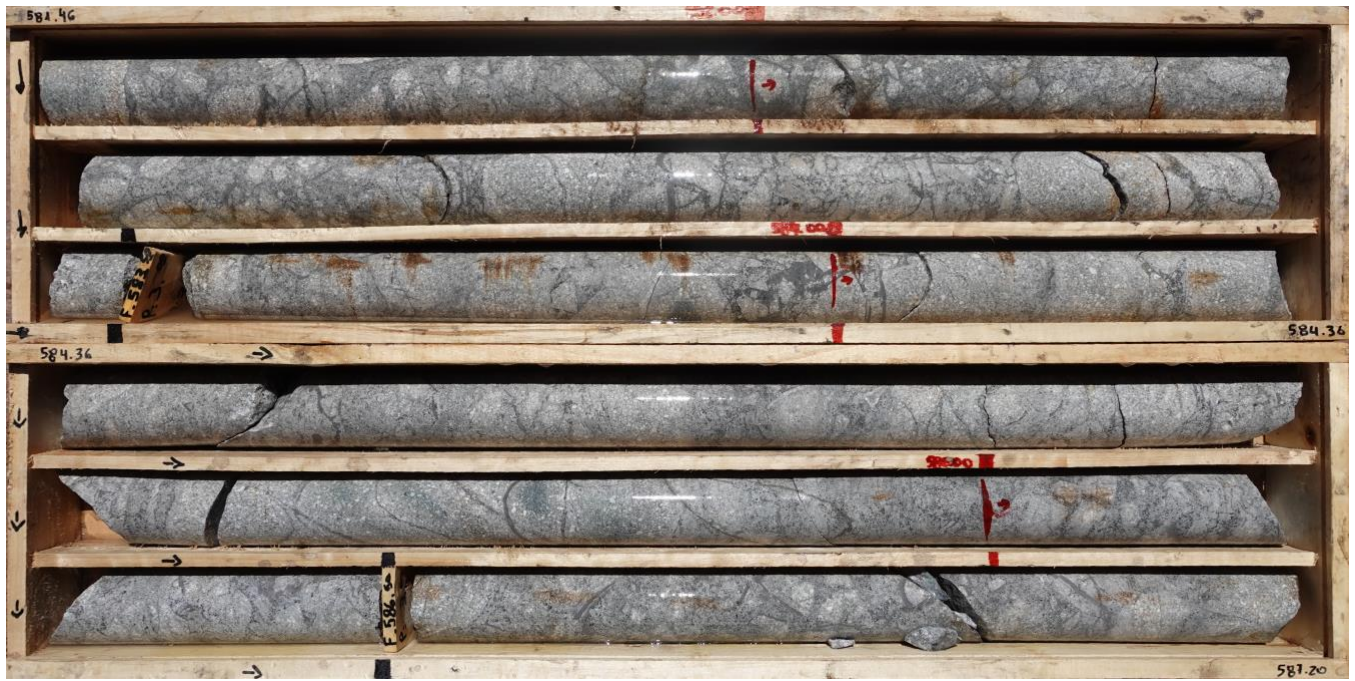
Image 3. 581.46 – 587.20. Hydrothermal breccia cutting diorite porphyry and containing clasts of early formed porphyry-style A veins.
