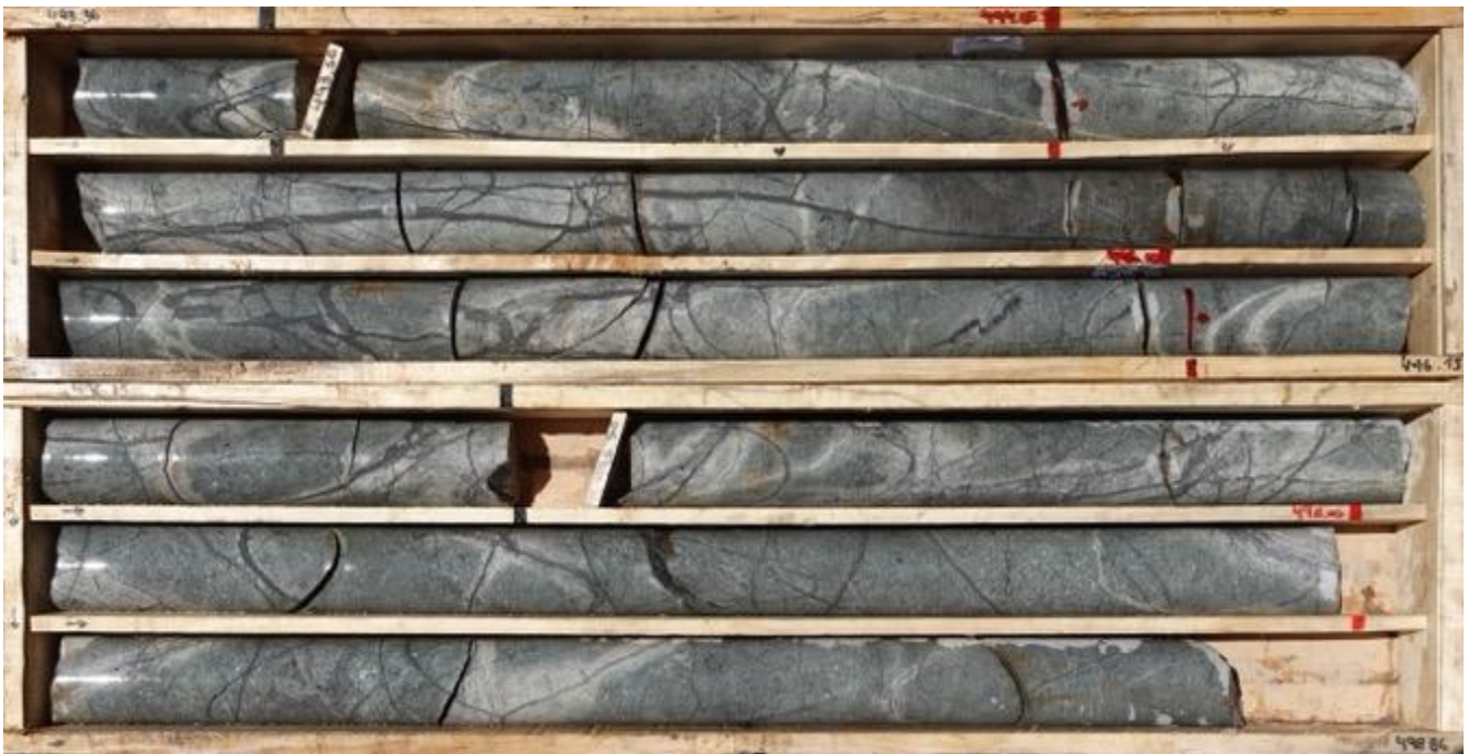
Image 2: 493.36 – 498.86m. Moderate intensity quartz-pyrite-chalcopyrite stockwork veining in diorite porphyry displaying early biotite potassic alteration overprinted by sericite-pyrite phyllic alteration.
