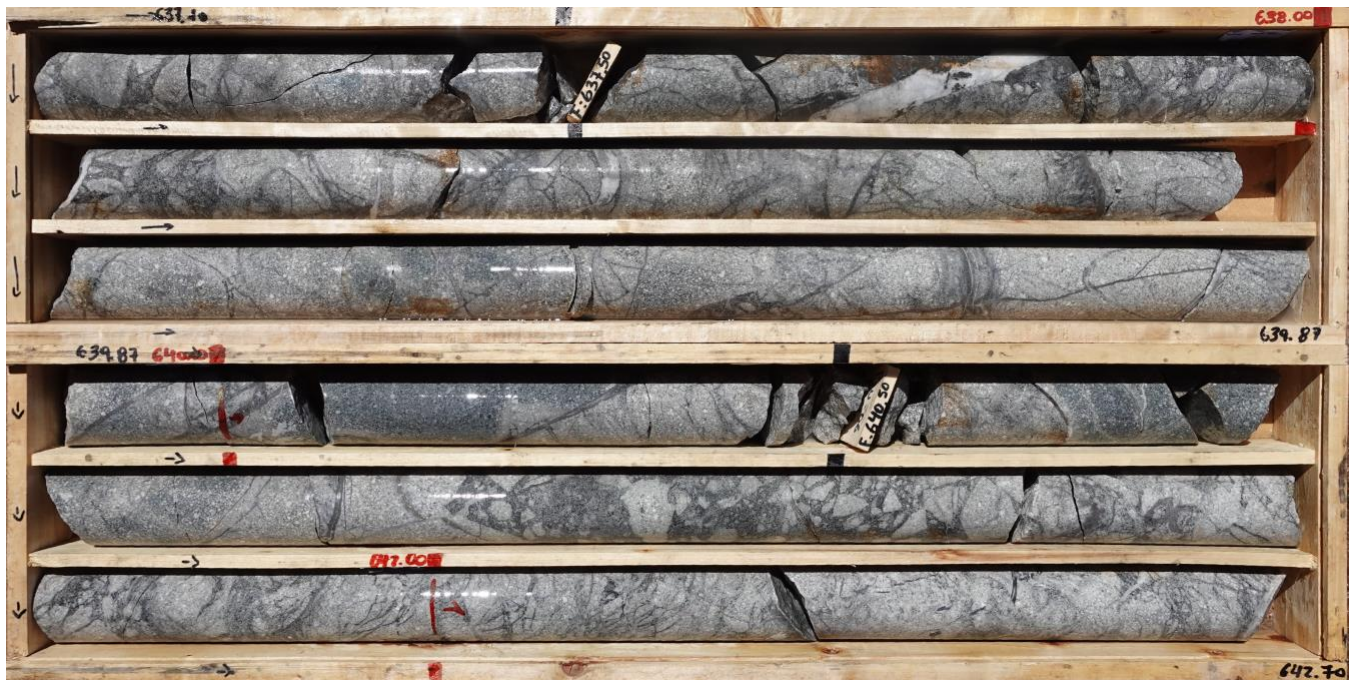
Image 4. 637.10 – 642.70. Hydrothermal breccia cutting diorite porphyry and containing clasts of early formed porphyry-style A veins.
