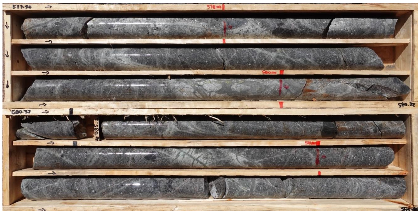
Image 1: PIU-05 577.5 - 583.16m. Strongly veined porphyry and diorite host rock and intercalated quartz-porphyry, showing multiphase quartz A-veins and associated K-feldspar bearing potassic alteration.
