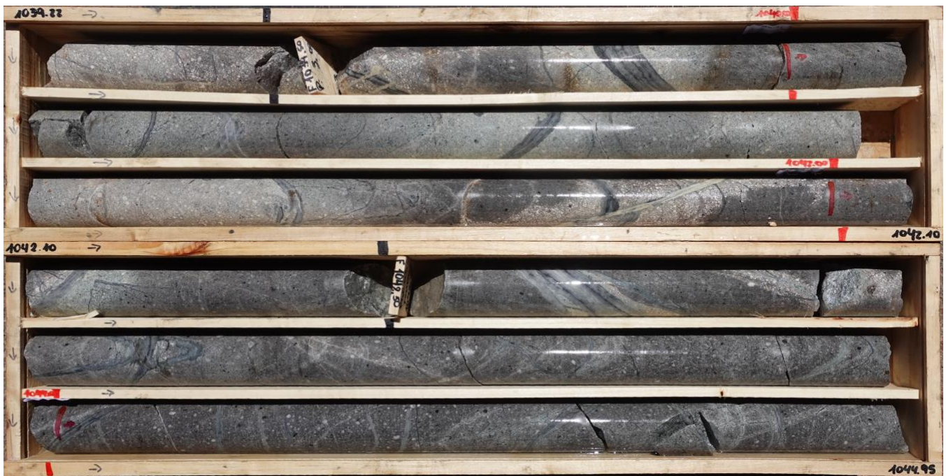
Image 3: PIU-05 1039.22 - 1044.95m. Distinct banded quartz-magnetite-pyrite vein phase hosted by intermineral porphyry and pre-mineral host rock intrusion.
