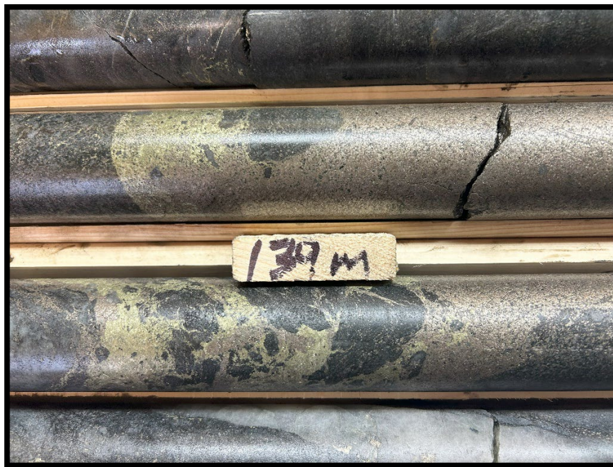
Photo 9. Massive sulphide core – PTX's drill hole W224-03.
