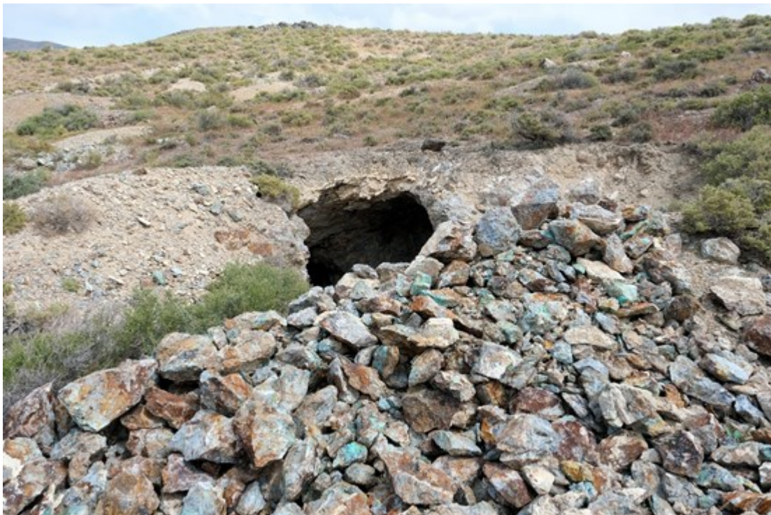
Figure 2: A Star South adit showing green malachite (copper) mineralization dump rocks
