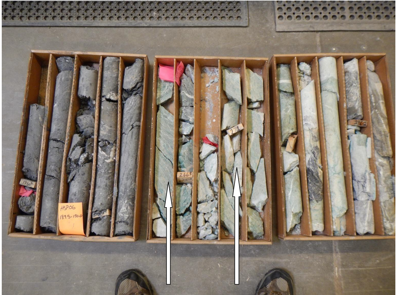
Figure 4a Fuchsite-Listwanite altered mafic dike containing chromium (884 ppm), nickel (639 ppm) and mercury (21 ppm) Doe Run Core Hole HSP-05-06. X-ray mineral identification not completed.
