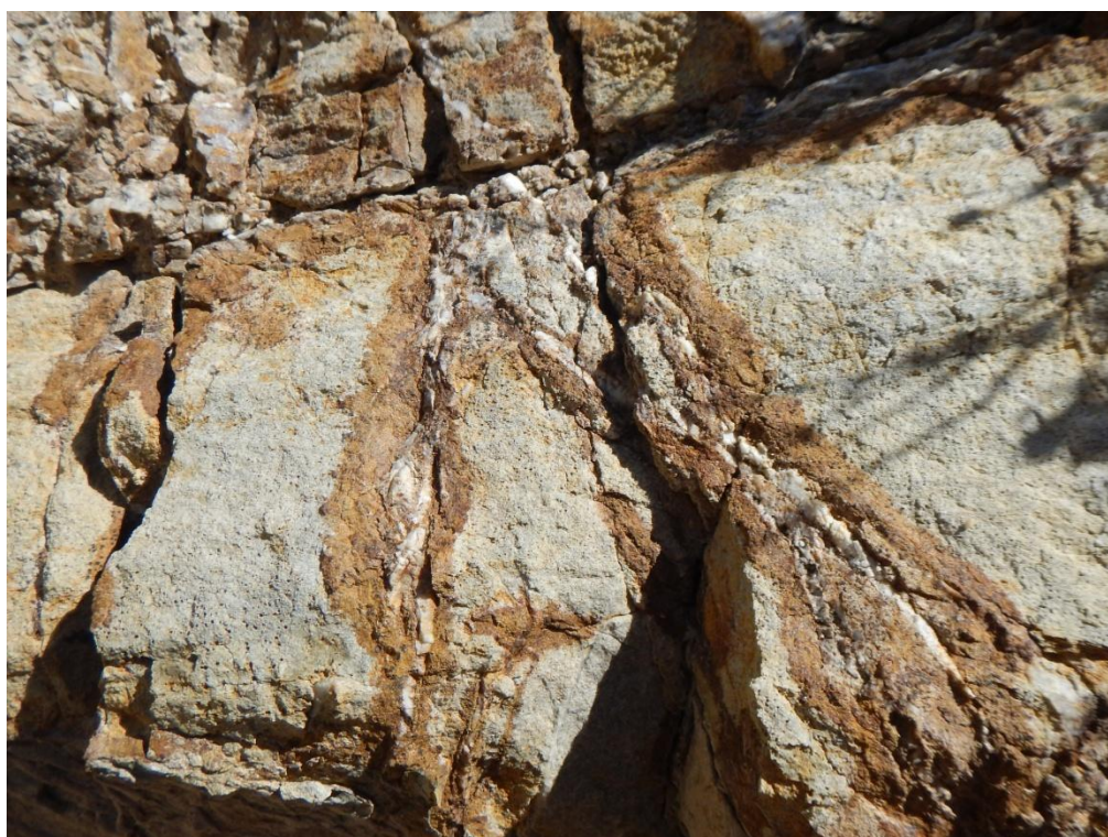
Figure 4f A second vein type containing quartz-limonite veins surrounded by coarse sericite-muscovite reaction rims, further altering the surrounding hornfels.
