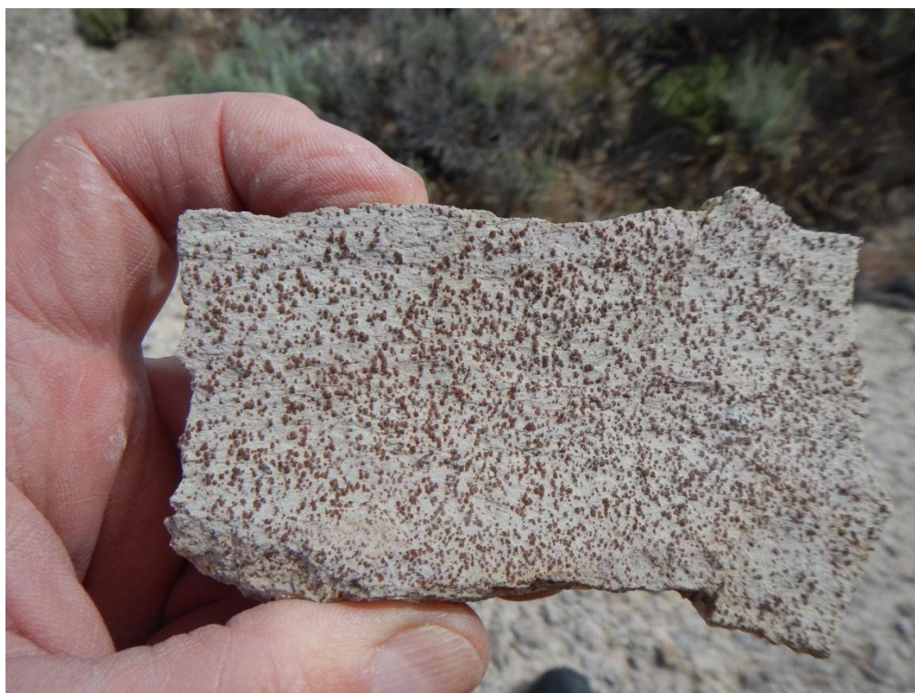
Figure 4e Spotted hornfels altered calcareous sandstone host rock in the mine area
