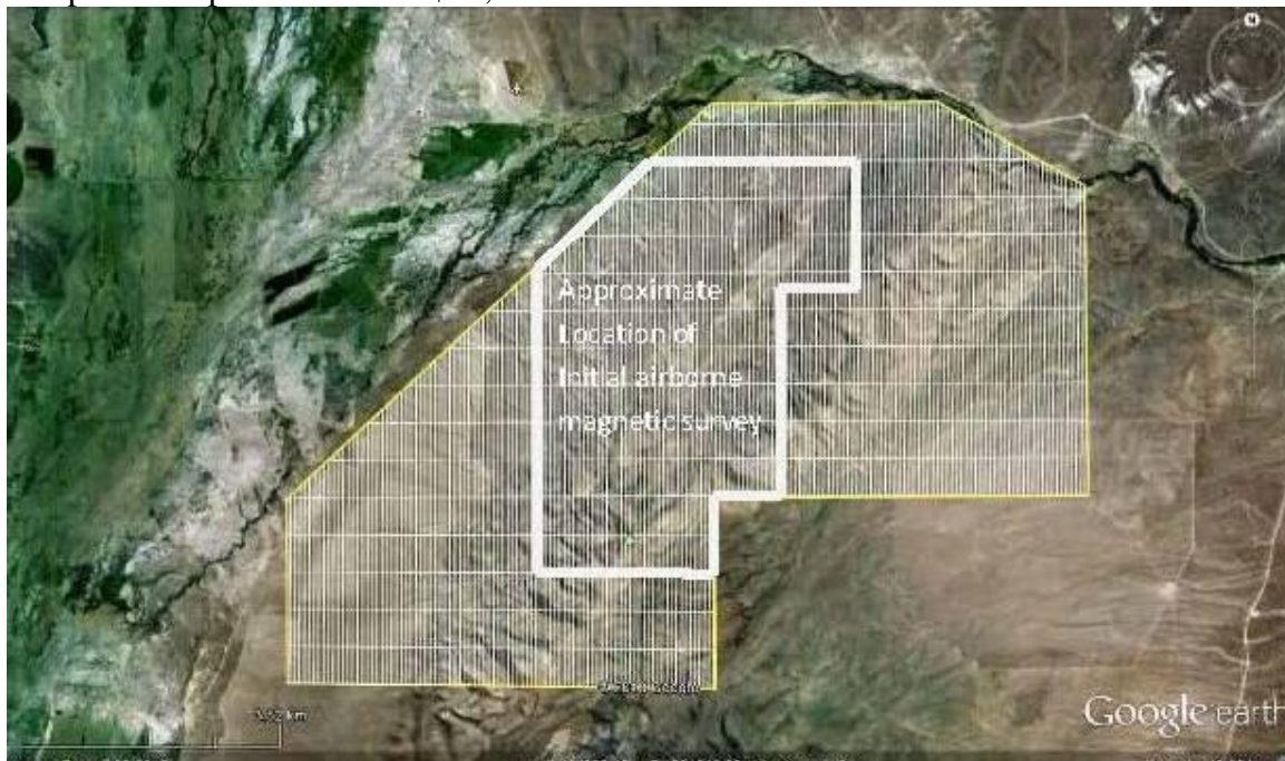
Figure 11 Airborne magnetic survey plan for the Hot Springs Peak Project showing flight-line density of 50 meters with cross connector lines at wider spacing.
