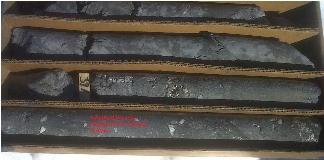
Figure 4b Carbon rich breccia with silicified fragments in Doe Run core hole HSP-05-06
