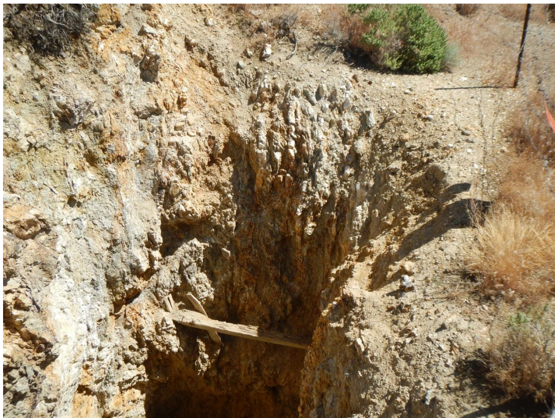
Figure 4c Shaft in the AMAX Area sunk on vertical quartz veined breccia zone
