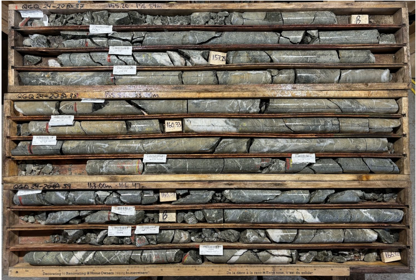
Figure 5: Core photo of bleached volcanics with quartz-carbonate-pyrite veins from 155.20 to 166.42 m in drill hole QGQ24-20
