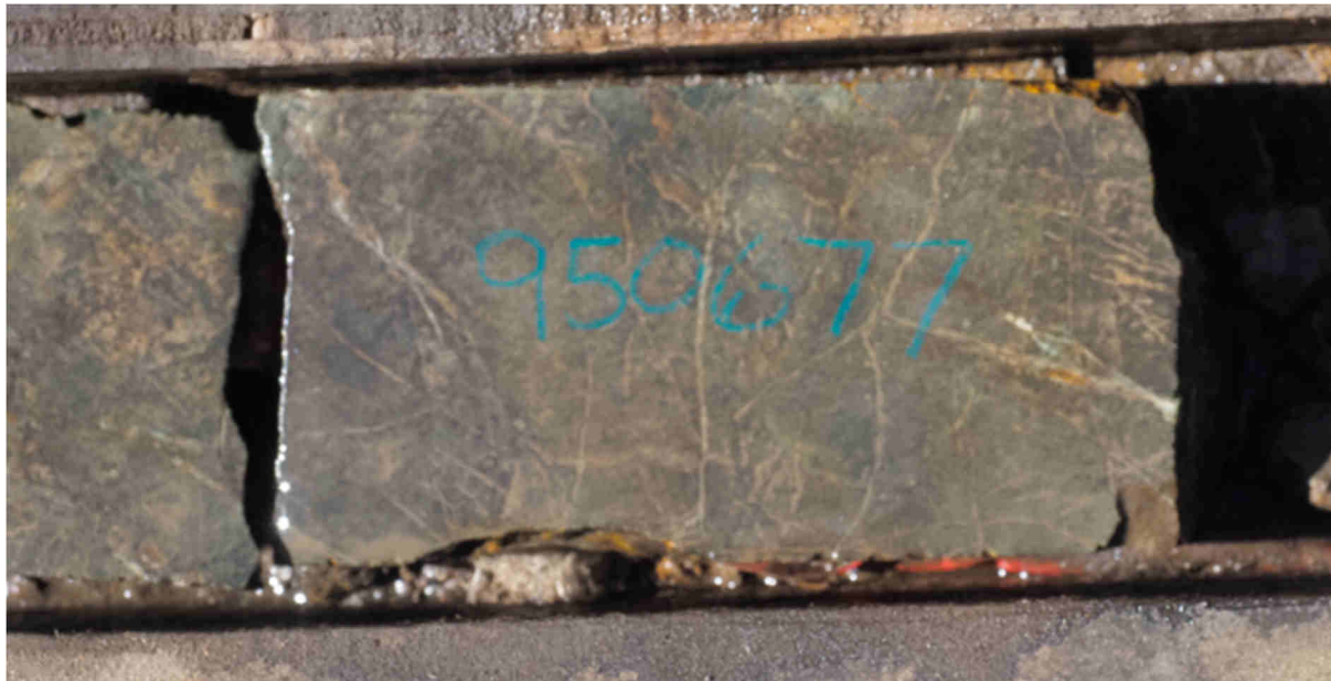
Figure 12-6 – K-SILICATE ALTERATION IN MAFIC FLOW (HOLE 11052)
